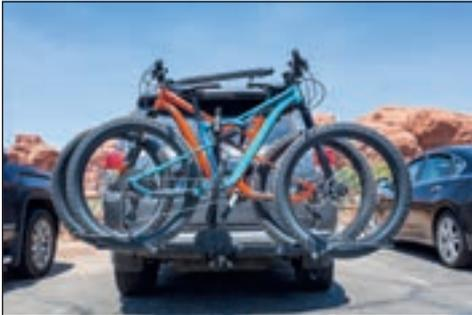
A bicycle carrier mounted on a tow bar.
