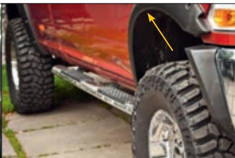
Tyres may not protrude more than three centimetres from the wheel arches (wheel arch is indicated by the arrow).
