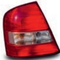
*With passenger cars, these retro-reflectors are usually incorporated in the light fixtures (in the same sections as the head and rear lights).*
