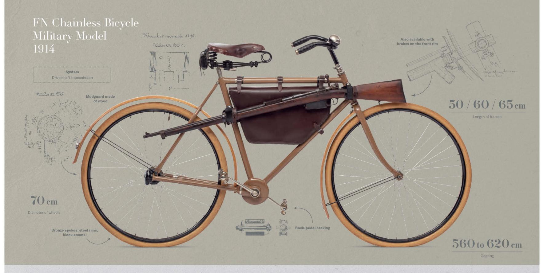
In 1898, FN developed its own **chainless system**, or **acatène**, bicycle, with a shaft-drive. The replacement of the chain by bevel gears was a major development for bicycles. The design of the drive system helped to distribute the forces more efficiently. The force applied to the pedals was transmitted by the cranks, the axle and the drive sprocket to a 17-tooth bevel gear, which was
