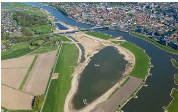
In accordance with the national plan Ruimte voor de rivier (2007), the dimensions of the IJssel's riverbed at Deventer have been adapted to climate change.
