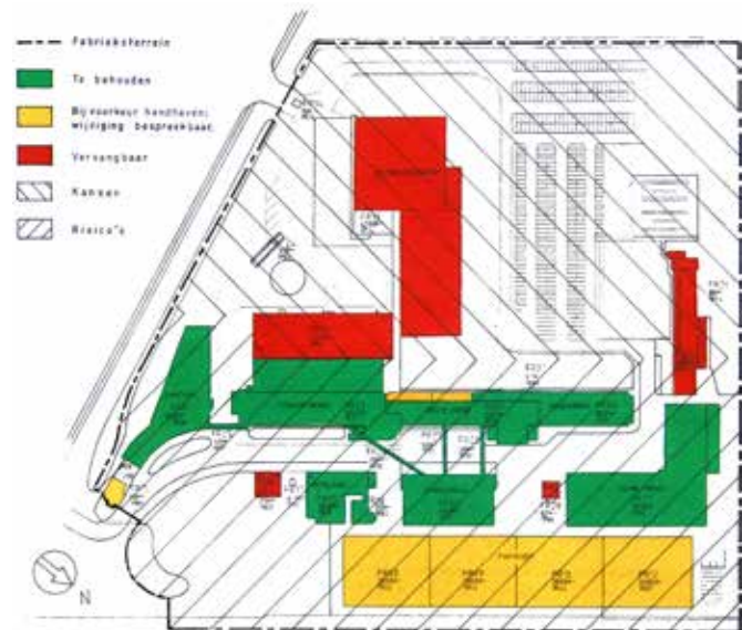
FIG. 5.11 A map from the 1998 Cultural Historic Reconnaissance for the Van Nelle Factory indicating the ‘opportunities’ and ‘challenges’ for redevelopment. This was composed to provide for a level playing field for commercial parties on which to base their respective bids / Rijksdienst voor het Cultureel Erfgoed
