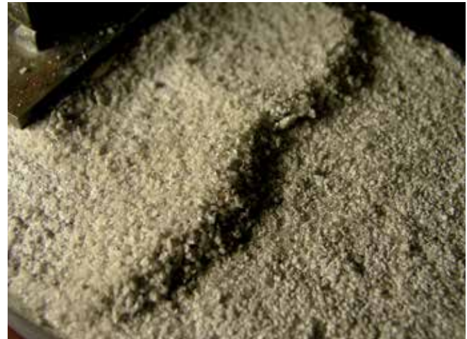
FIG. 7.7 Sanding of the outer layer of the mortar in the presence of NaCl after 6 RH cycles / photo: s Barbara Lubelli
