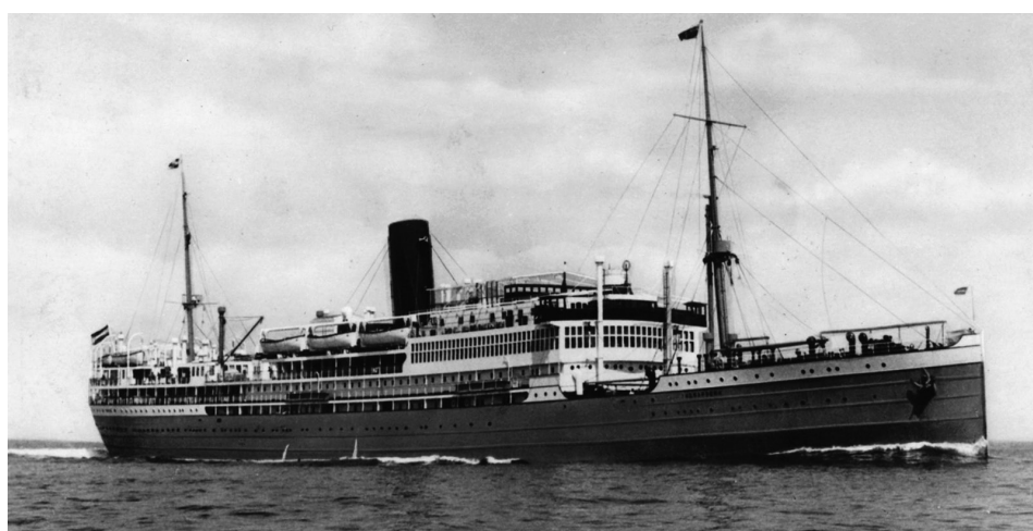
ss Indrapoera (1926-1956; 10.825 gross). In 1932 lengthened at the Schelde dockyard and equipped with diesel engines. Her beautiful interiors were destroyed in 1940 when she became a troop transport. In 1949 converted into a freight/passenger ship.
