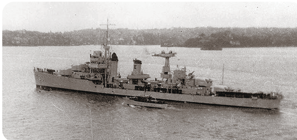
USS Clark entering port in 1941. The ships of the Porter- and Somers class were quite badly overweighted. During WW2 they were rebuilt with dual-purpose guns and their Mk 35 directors refurbished.
