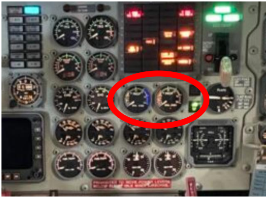
Figure 2: Saab SF340B engine indications
