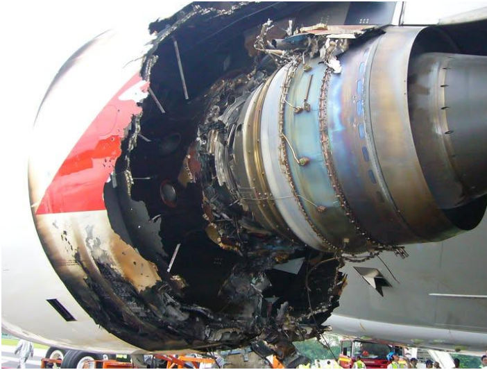
Figure 5: The failed Rolls-Royce Trent 900 engine of QF32
