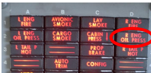
Figure 1: Saab SF340B Central Warning Panel indications
