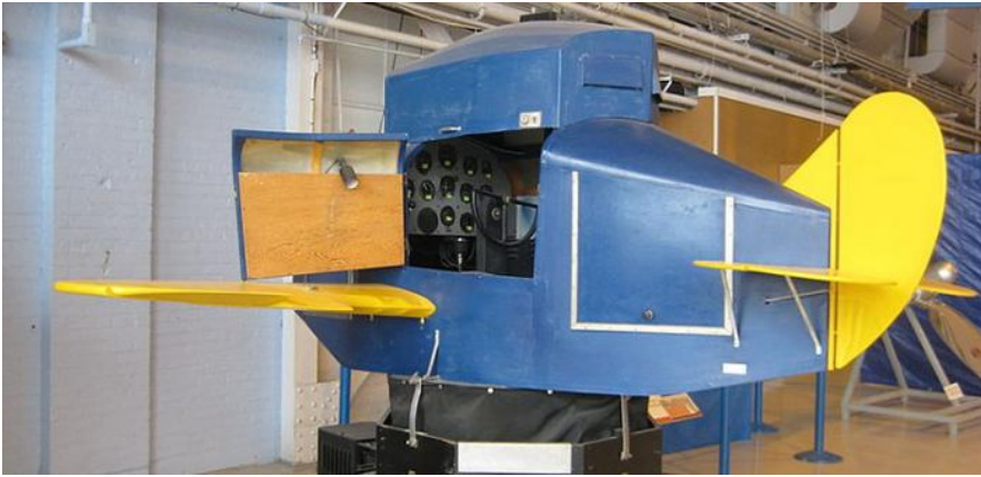
Figure 12: The Link Trainer, the world's first commercial flight simulator
