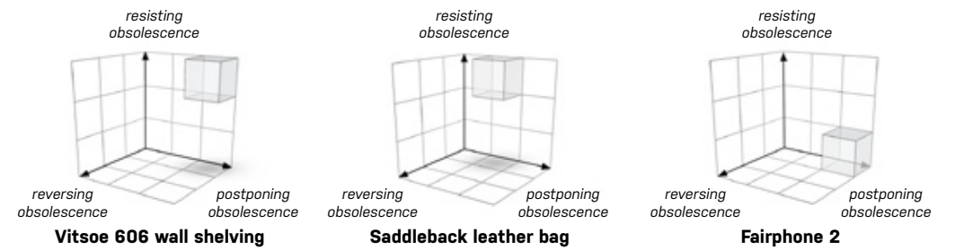
Figure S.2: Example products plotted in the three-dimensional design space for preserving product integrity. The three dimensions are formed by the three design directions for preserving product integrity: resisting obsolescence, postponing obsolescence and reversing obsolescence.
