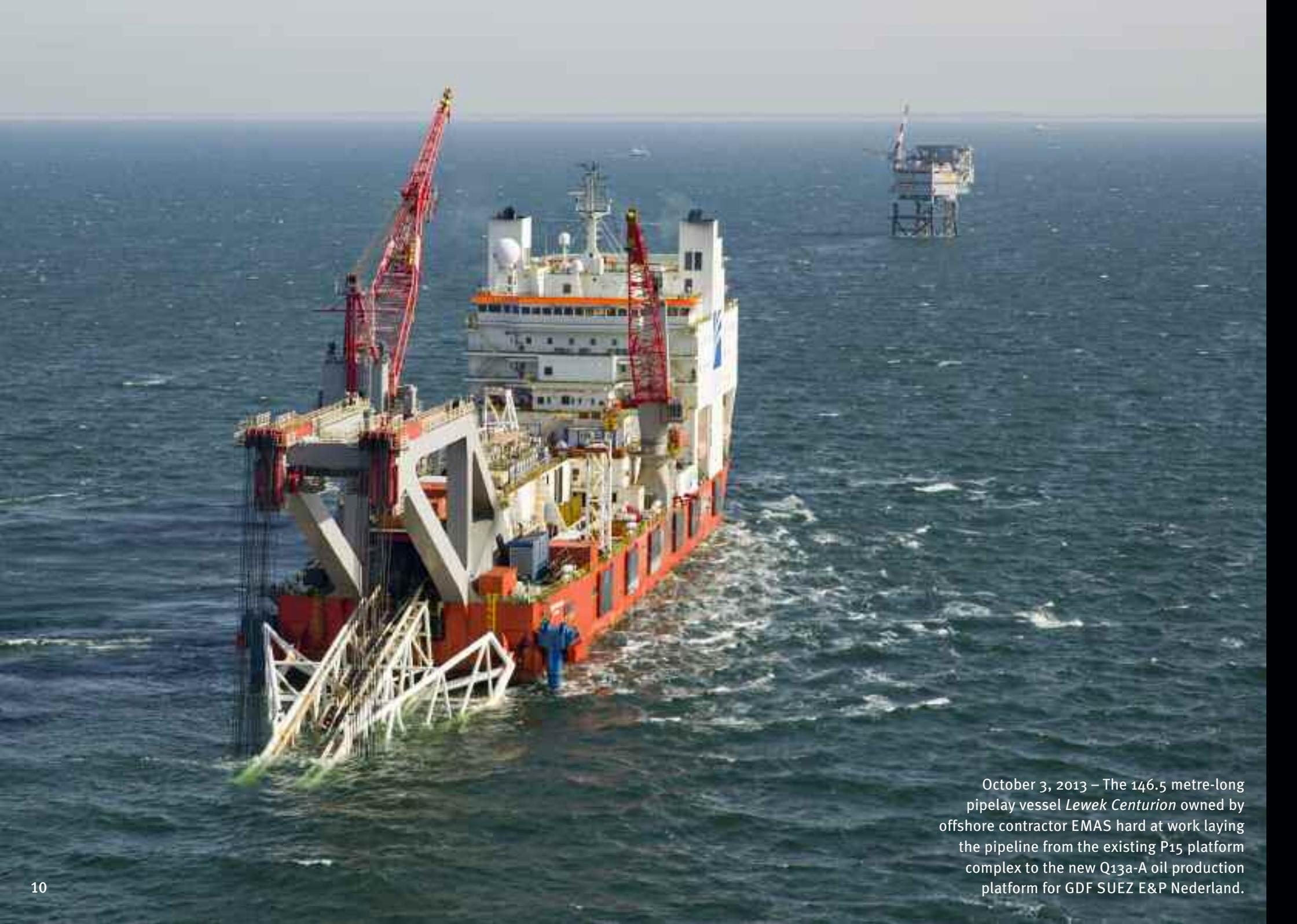
October 3, 2013 – The 146.5 metre-long pipelay vessel *Lewek Centurion* owned by offshore contractor EMAS hard at work laying the pipeline from the existing P15 platform complex to the new Q13a-A oil production platform for GDF SUEZ E&P Nederland.
