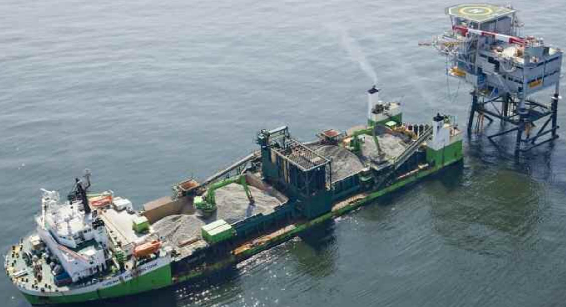
July 22, 2013 – The dp2 fall pipe vessel *Tideway Rollingstone* from Tideway was deployed to prevent scouring of the seabed around the new Q13a-A platform operated by GDF SUEZ E&P Nederland. The 139 metre-long *Rollingstone* has a payload of almost 12,000 tonnes of rock for dumping.
