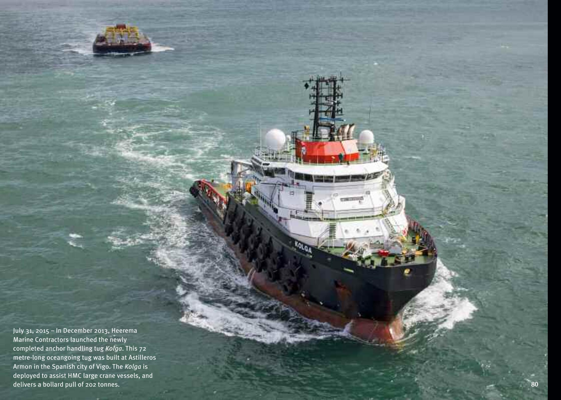
July 31, 2015 – In December 2013, Heerema Marine Contractors launched the newly completed anchor handling tug *Kolga*. This 72 metre-long oceangoing tug was built at Astilleros Armon in the Spanish city of Vigo. The *Kolga* is deployed to assist HMC large crane vessels, and delivers a bollard pull of 202 tonnes.
