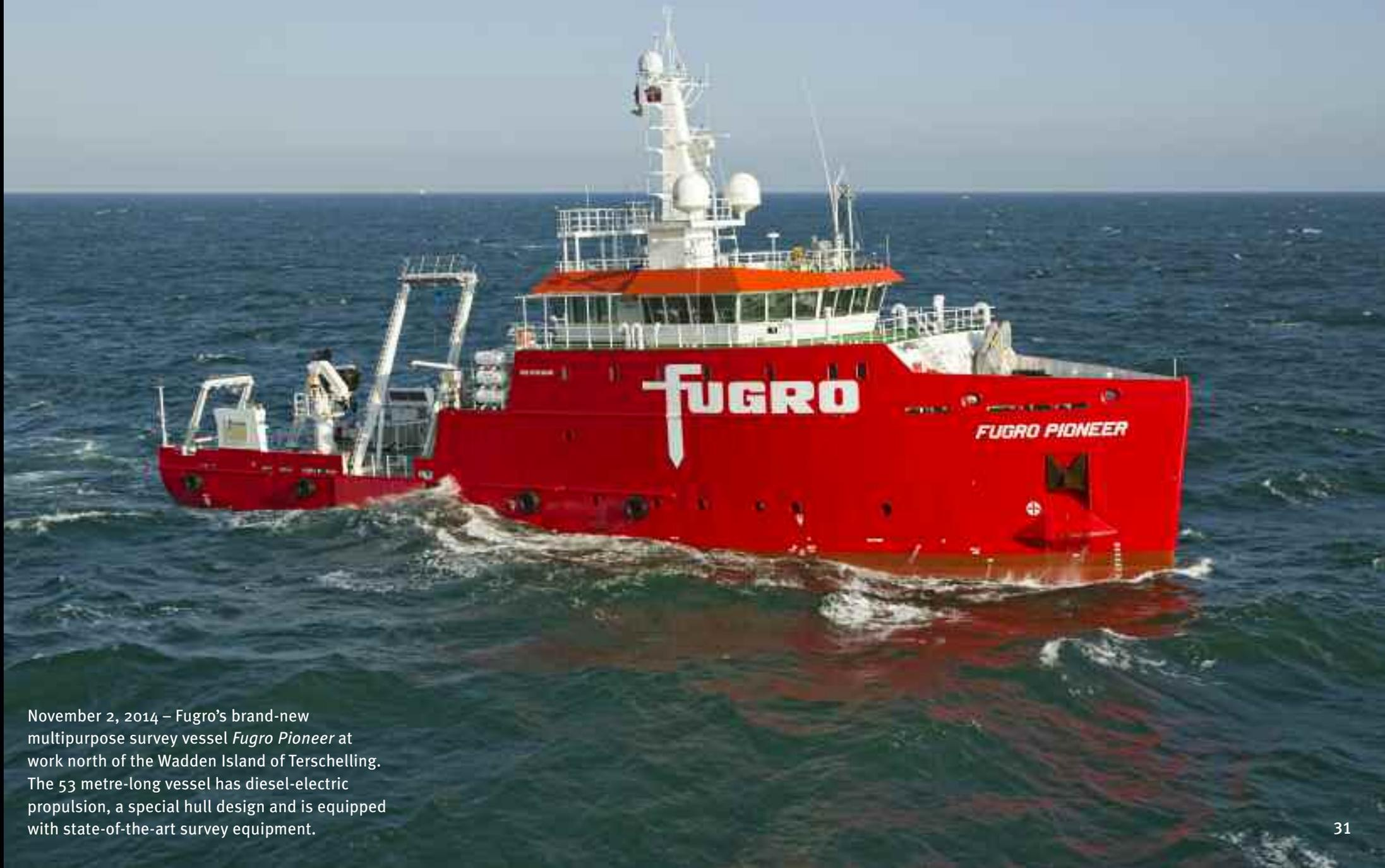
November 2, 2014 – Fugro’s brand-new multipurpose survey vessel *Fugro Pioneer* at work north of the Wadden Island of Terschelling. The 53 metre-long vessel has diesel-electric propulsion, a special hull design and is equipped with state-of-the-art survey equipment.
