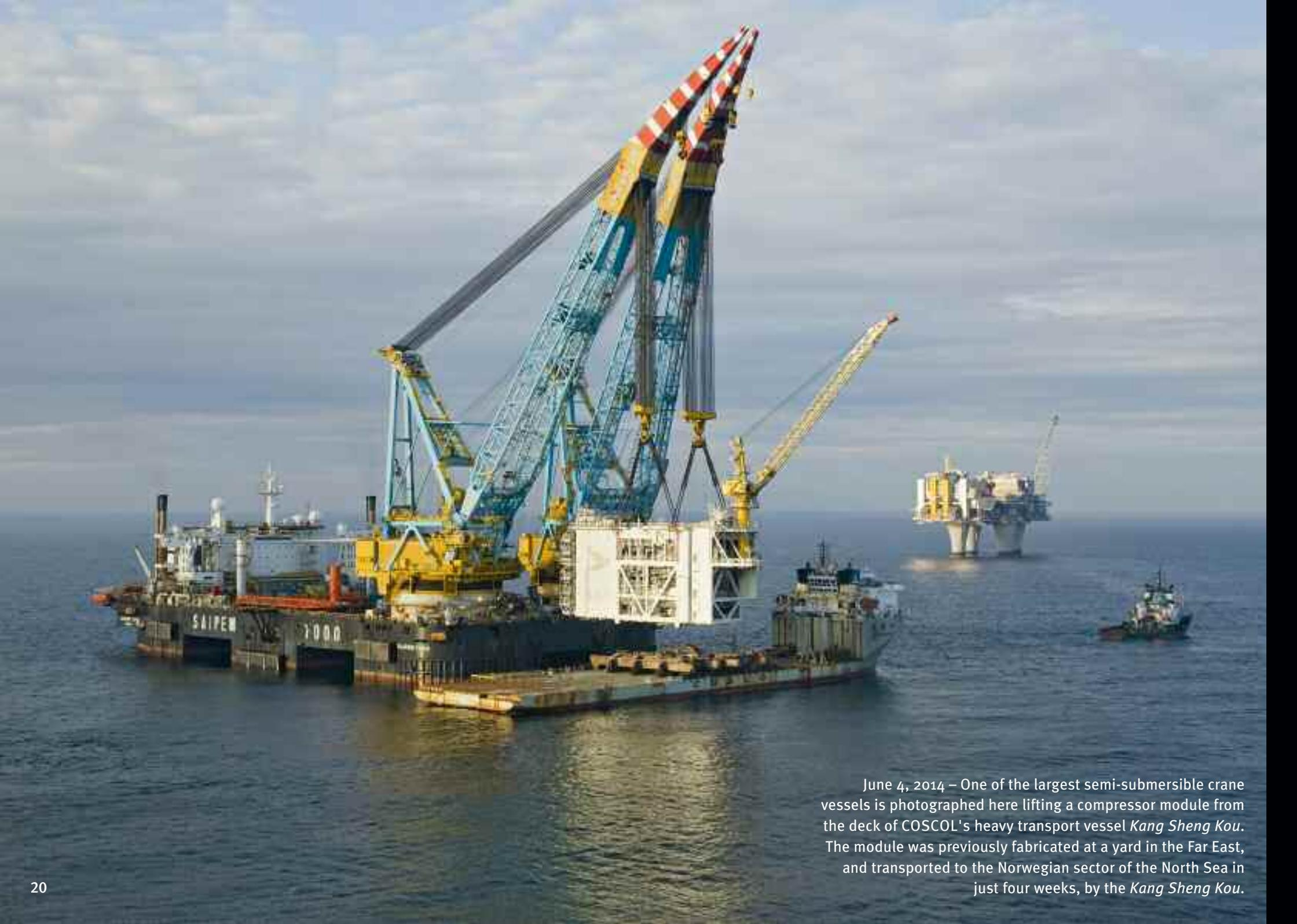
June 4, 2014 – One of the largest semi-submersible crane vessels is photographed here lifting a compressor module from the deck of COSCOL's heavy transport vessel *Kang Sheng Kou*. The module was previously fabricated at a yard in the Far East, and transported to the Norwegian sector of the North Sea in just four weeks, by the *Kang Sheng Kou*.
