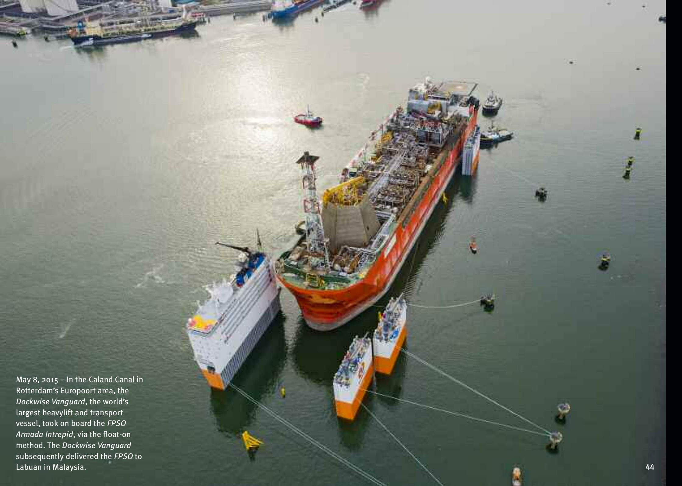
May 8, 2015 – In the Caland Canal in Rotterdam’s Europoort area, the *Dockwise Vanguard*, the world’s largest heavylift and transport vessel, took on board the *FPSO Armada Intrepid*, via the float-on method. The *Dockwise Vanguard* subsequently delivered the *FPSO* to Labuan in Malaysia.
