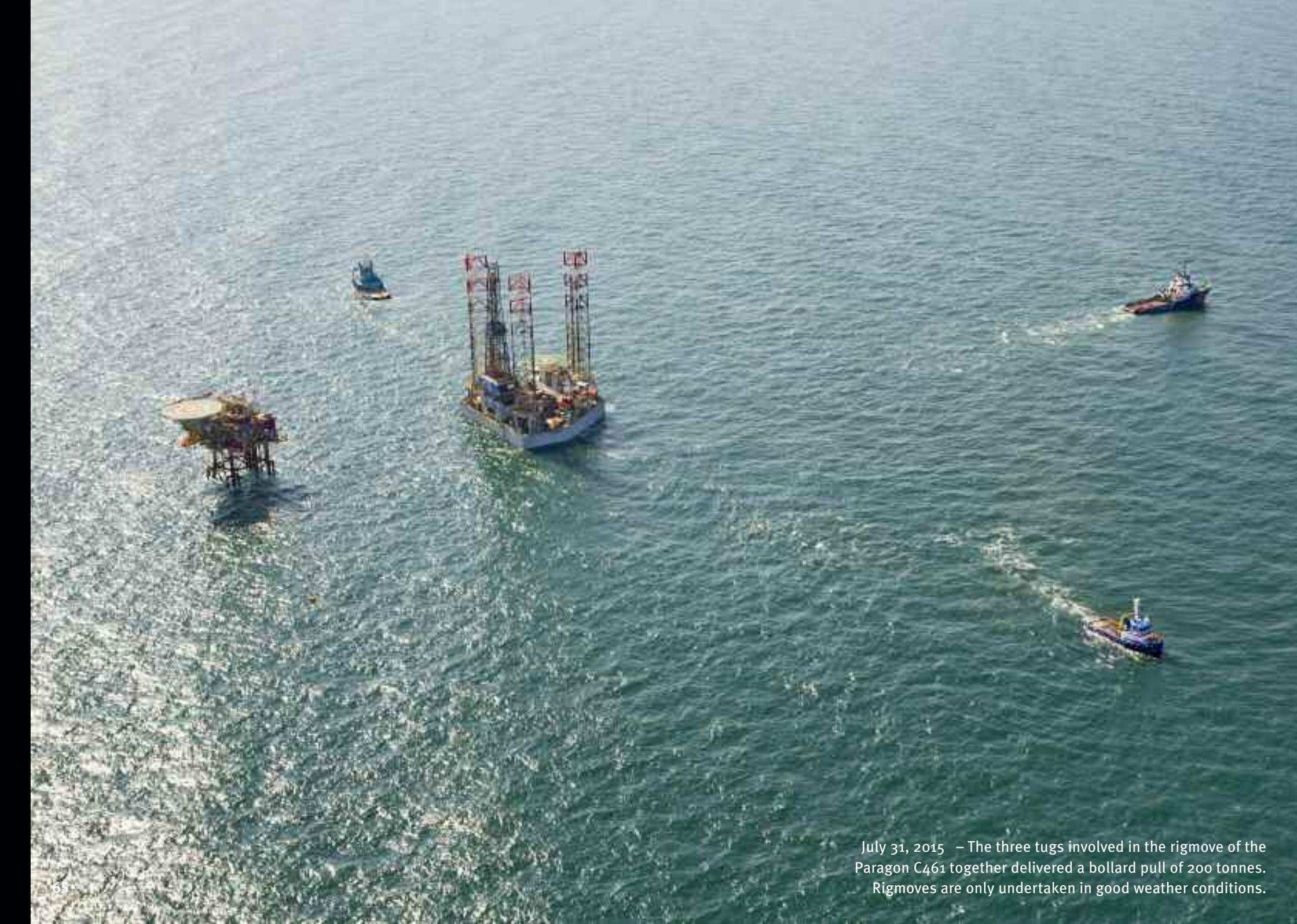
July 31, 2015 – The three tugs involved in the rigmove of the Paragon C461 together delivered a bollard pull of 200 tonnes. Rigmoves are only undertaken in good weather conditions.
