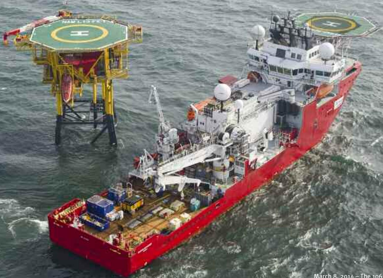
March 8, 2014 – The 106 metre-long diving support vessel *Skandi Achiever* operated by French contractor Technip is seen here working at NAM's L13-FE-1 satellite platform in the Dutch sector of the North Sea. The platform is used for the production of gas from the L13 block.
