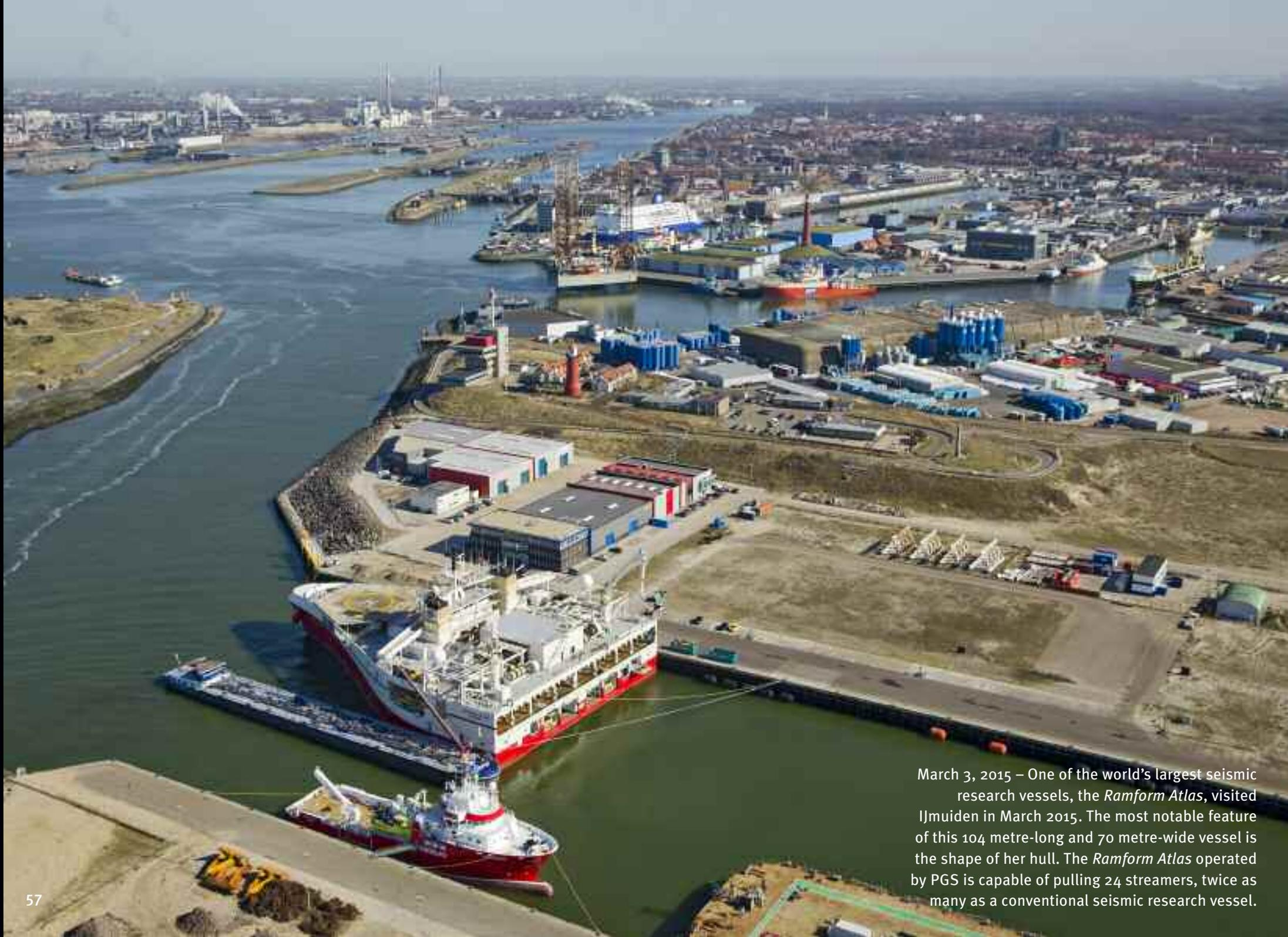
March 3, 2015 – One of the world's largest seismic research vessels, the *Ramform Atlas*, visited IJmuiden in March 2015. The most notable feature of this 104 metre-long and 70 metre-wide vessel is the shape of her hull. The *Ramform Atlas* operated by PGS is capable of pulling 24 streamers, twice as many as a conventional seismic research vessel.
