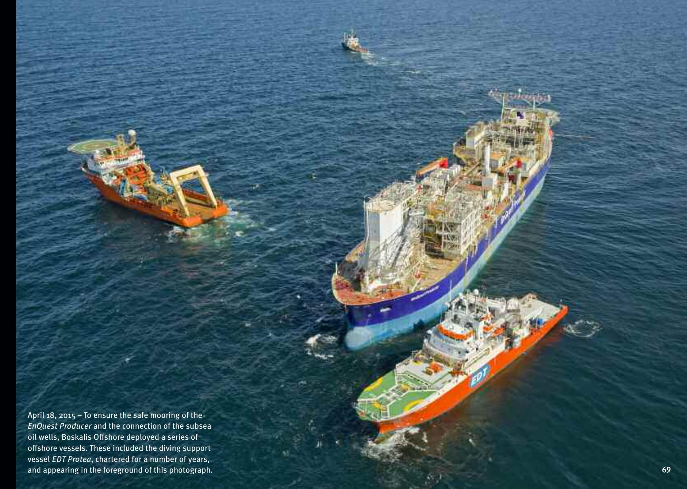
April 18, 2015 – To ensure the safe mooring of the *EnQuest Producer* and the connection of the subsea oil wells, Boskalis Offshore deployed a series of offshore vessels. These included the diving support vessel *EDT Protea*, chartered for a number of years, and appearing in the foreground of this photograph.
