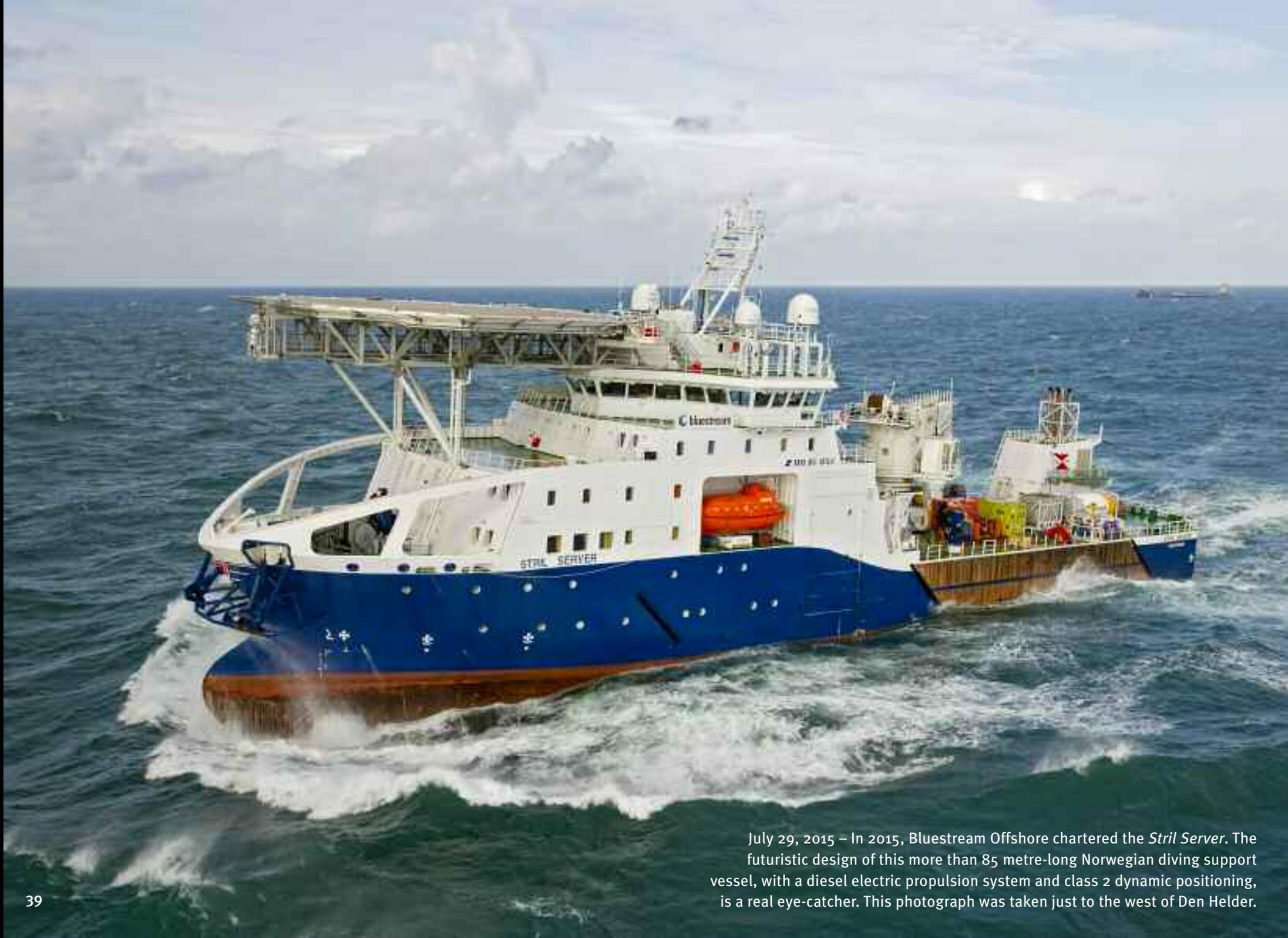
July 29, 2015 – In 2015, Bluestream Offshore chartered the *Stril Server*. The futuristic design of this more than 85 metre-long Norwegian diving support vessel, with a diesel electric propulsion system and class 2 dynamic positioning, is a real eye-catcher. This photograph was taken just to the west of Den Helder.
