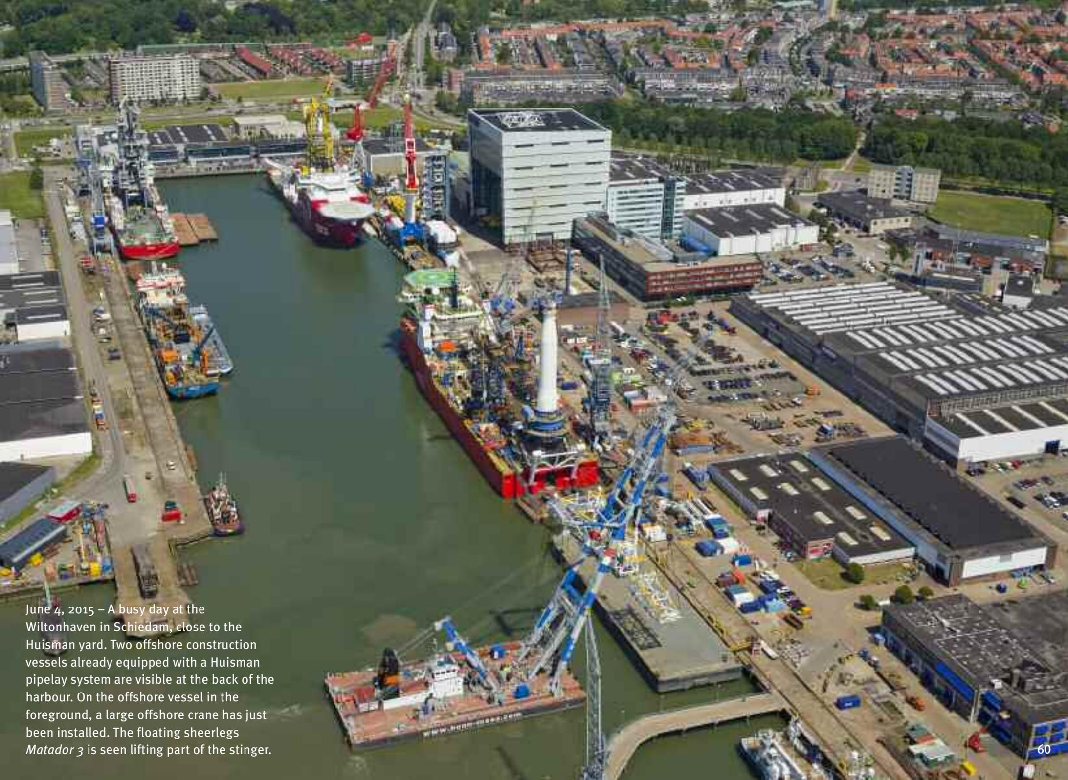
June 4, 2015 – A busy day at the Wiltonhaven in Schiedam, close to the Huisman yard. Two offshore construction vessels already equipped with a Huisman pipelay system are visible at the back of the harbour. On the offshore vessel in the foreground, a large offshore crane has just been installed. The floating shearlegs *Matador 3* is seen lifting part of the stinger.
