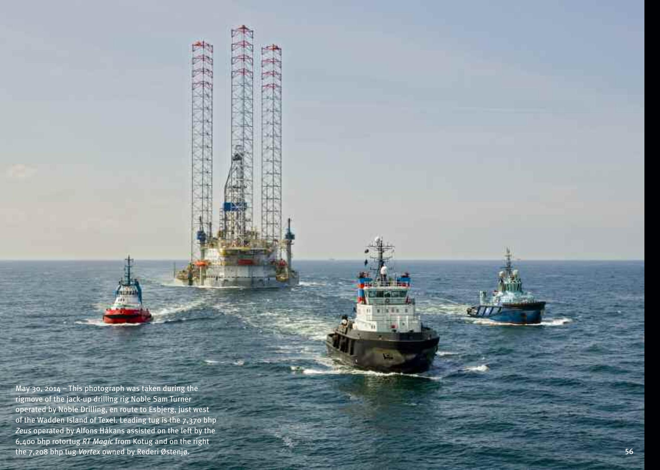
May 30, 2014 – This photograph was taken during the rigmove of the jack-up drilling rig Noble Sam Turner operated by Noble Drilling, en route to Esbjerg, just west of the Wadden Island of Texel. Leading tug is the 7,370 bhp Zeus operated by Alfons Håkans assisted on the left by the 6,400 bhp rotortug RT Magic from Kotug and on the right the 7,208 bhp tug Vortex owned by Rederi Østenjø.
