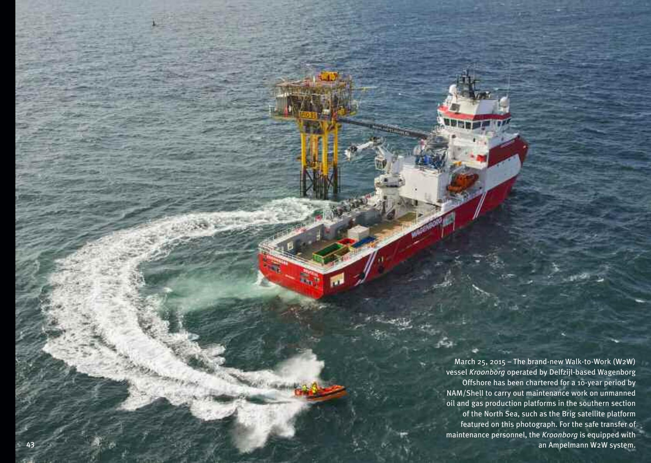
March 25, 2015 – The brand-new Walk-to-Work (W2W) vessel *Kroonborg* operated by Delfzijl-based Wagenborg Offshore has been chartered for a 10-year period by NAM/Shell to carry out maintenance work on unmanned oil and gas production platforms in the southern section of the North Sea, such as the Brig satellite platform featured on this photograph. For the safe transfer of maintenance personnel, the *Kroonborg* is equipped with an Ampelmann W2W system.
