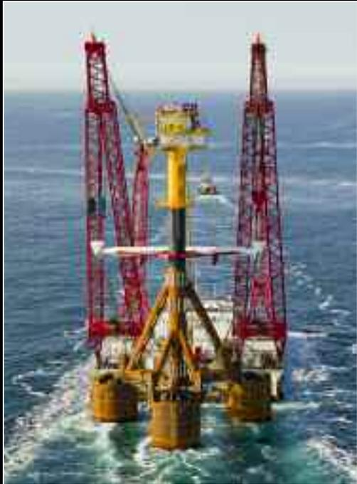
*Crane vessel Rambiz underway for an offshore installation.*
