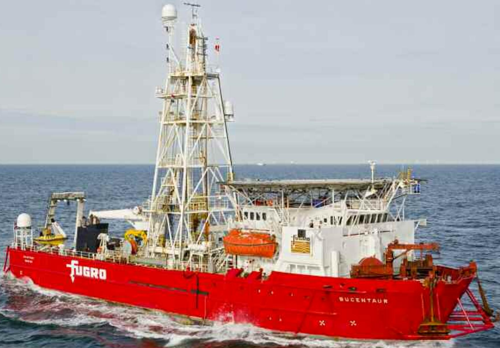
October 18, 2014 – At the end of 2014, Fugro Marine Services deployed its geotechnical drillship *Bucentaur* in the North Sea. On this photograph, the 77 metre-long vessel is seen sailing west of IJmuiden. The *Bucentaur* is able to carry out survey work to a maximum water depth of 1,500 metres.
