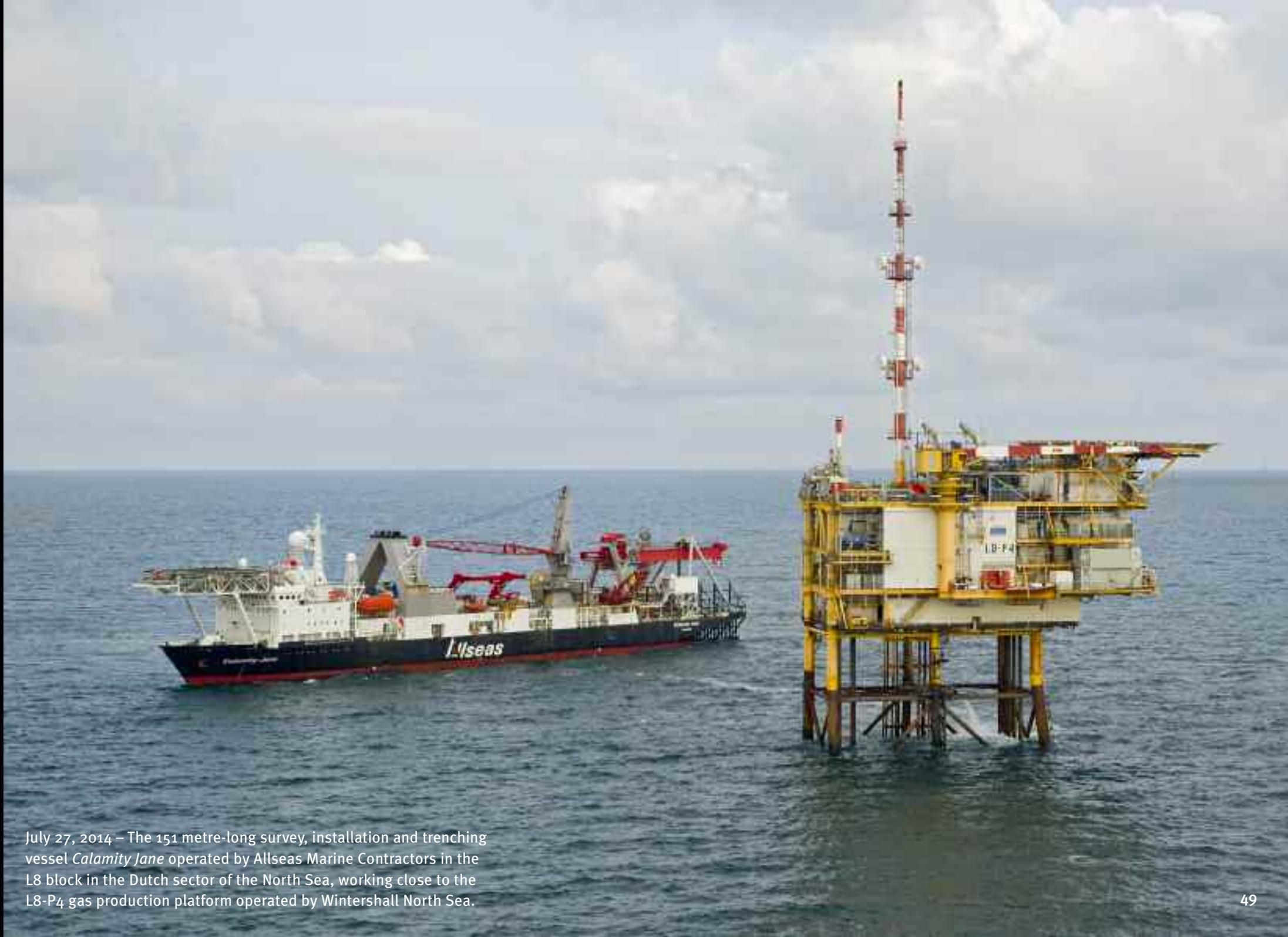
July 27, 2014 – The 151 metre-long survey, installation and trenching vessel *Calamity Jane* operated by Allseas Marine Contractors in the L8 block in the Dutch sector of the North Sea, working close to the L8-P4 gas production platform operated by Wintershall North Sea.
