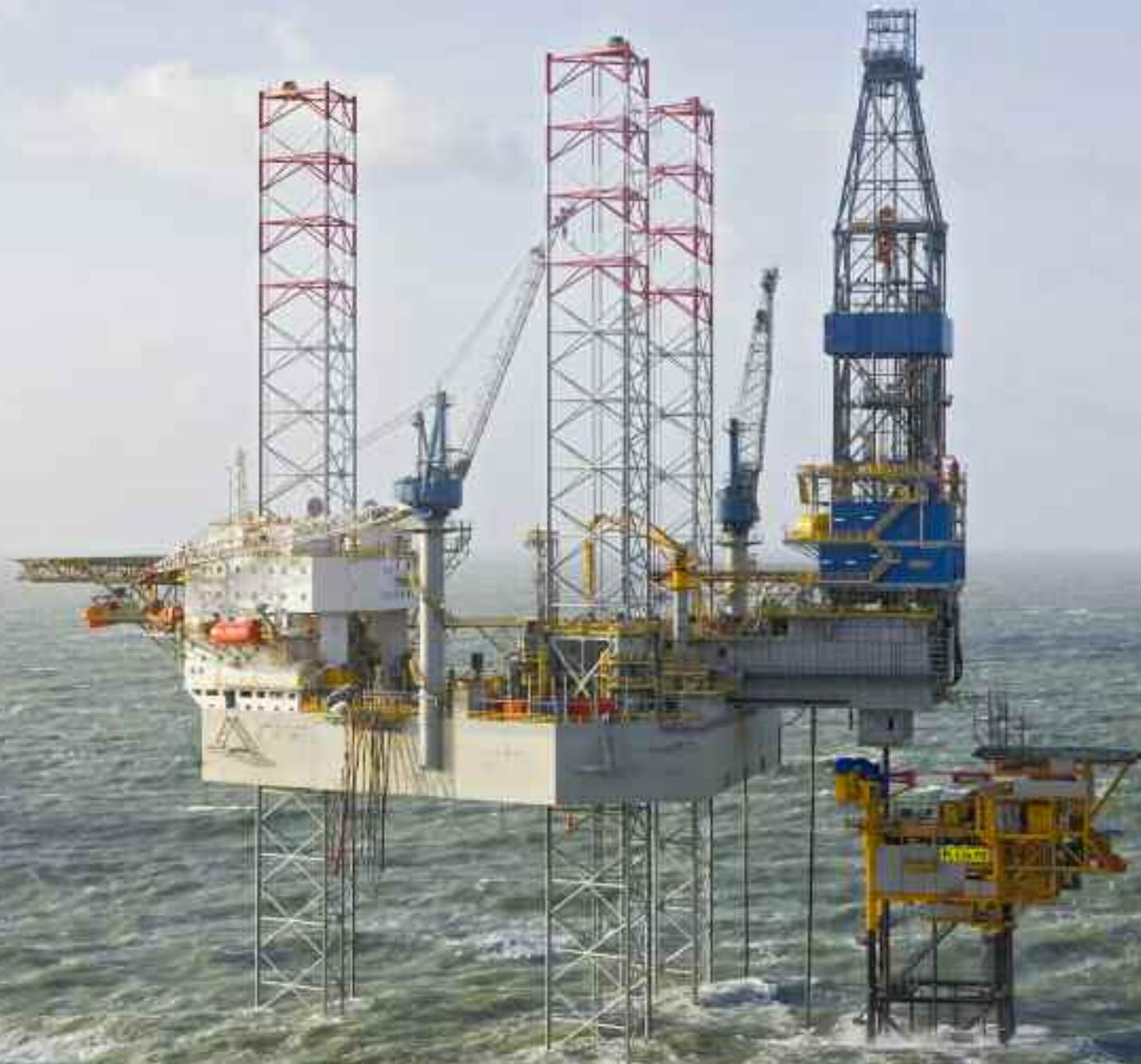
February 6, 2014 – The jack-up drilling rig Noble Regina Allen is photographed here drilling the first gas production wells for the GDF SUEZ E&P Nederland L5a-D gas production platform, just installed in the sea 45 miles northwest of the Wadden Island of Terschelling. The drilling rig is of the type Friede & Goldman JU3000N, and was fabricated at the Jurong Shipyard in Singapore.
