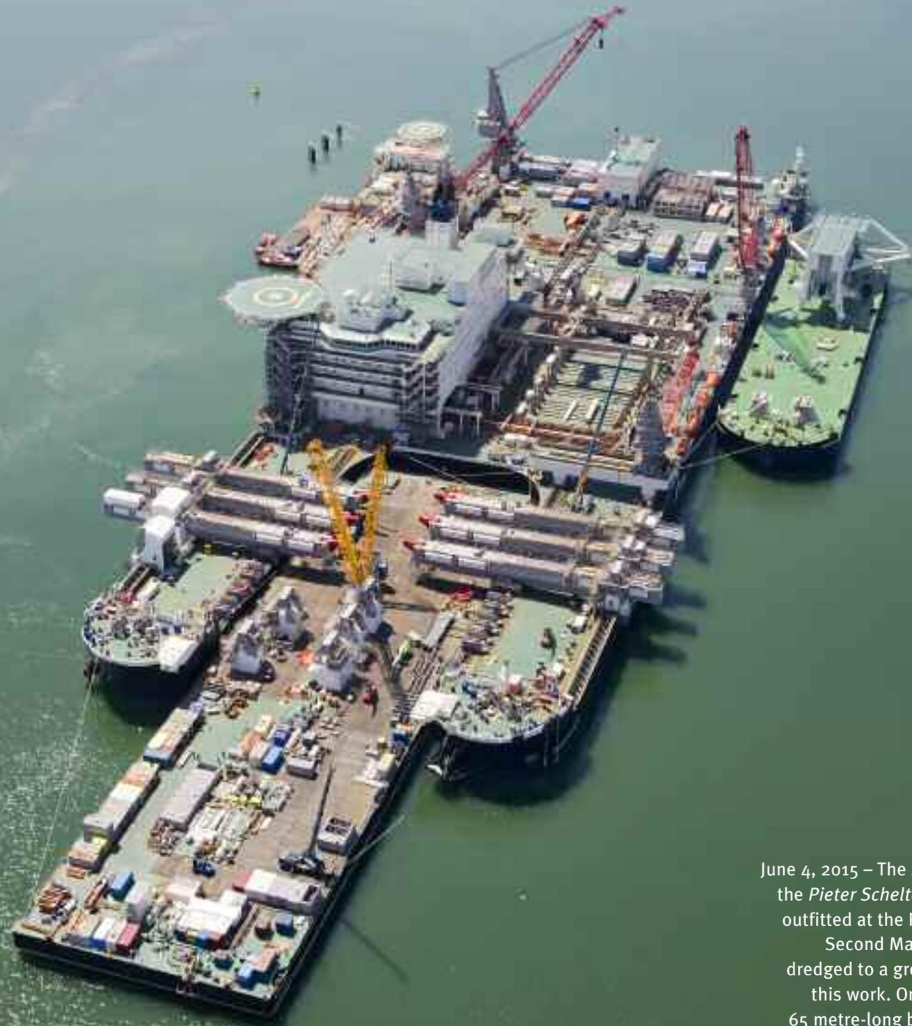
June 4, 2015 – The *Pioneering Spirit*, formerly the *Pieter Schelte*, owned by Allseas, being outfitted at the Prinses Alexiahaven on the Second Maasvlakte. The harbour was dredged to a greater depth specifically for this work. On this photograph, the first 65 metre-long beams of the lifting system are already installed on the foreship.
