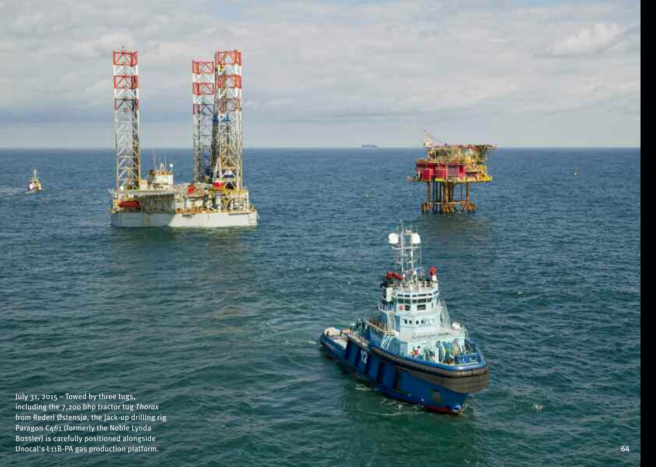
July 31, 2015 – Towed by three tugs, including the 7,200 bhp tractor tug *Thorax* from Rederi Østensjø, the jack-up drilling rig Paragon C461 (formerly the Noble Lynda Bossler) is carefully positioned alongside Unocal's L11B-PA gas production platform.
