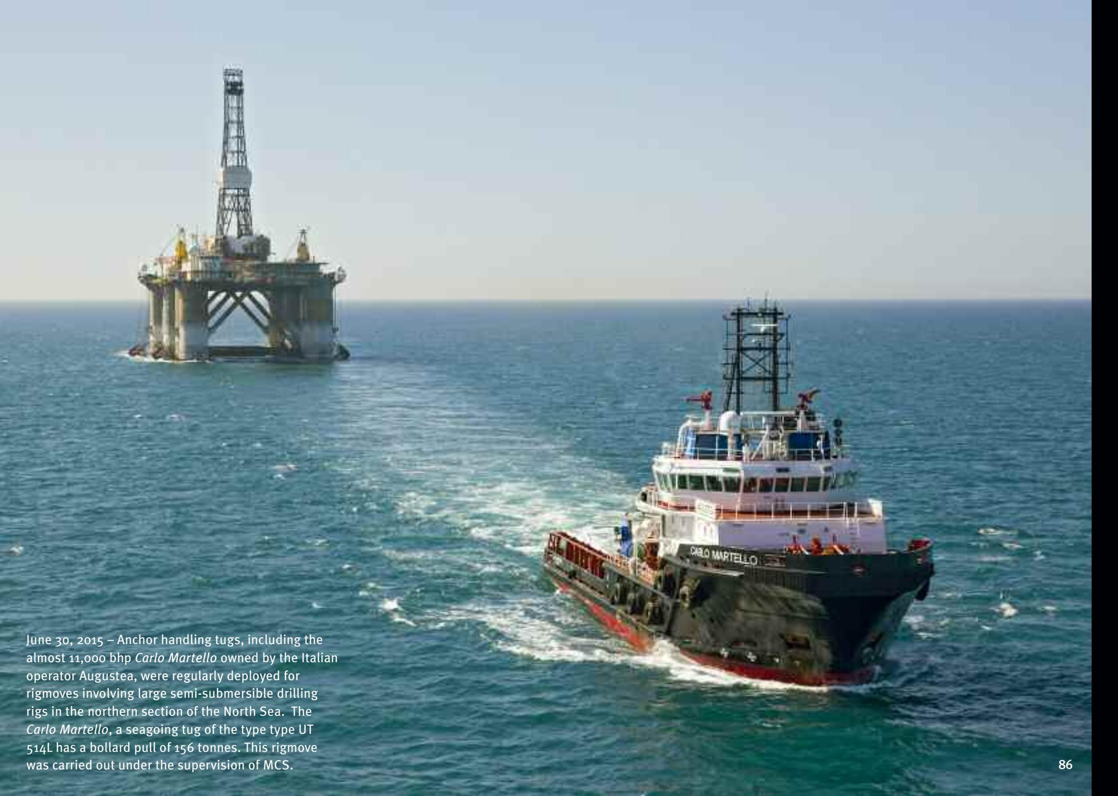
June 30, 2015 – Anchor handling tugs, including the almost 11,000 bhp *Carlo Martello* owned by the Italian operator Augustea, were regularly deployed for rigmoves involving large semi-submersible drilling rigs in the northern section of the North Sea. The *Carlo Martello*, a seagoing tug of the type type UT 514L has a bollard pull of 156 tonnes. This rigmove was carried out under the supervision of MCS.
