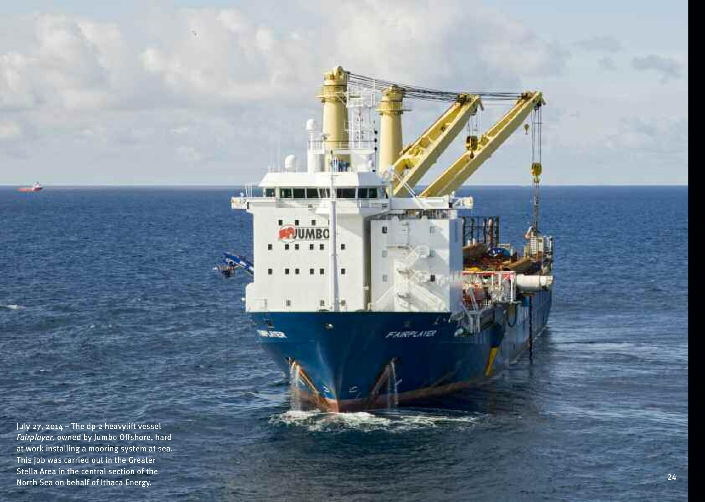
July 27, 2014 – The dp 2 heavylift vessel *Fairplayer*, owned by Jumbo Offshore, hard at work installing a mooring system at sea. This job was carried out in the Greater Stella Area in the central section of the North Sea on behalf of Ithaca Energy.
