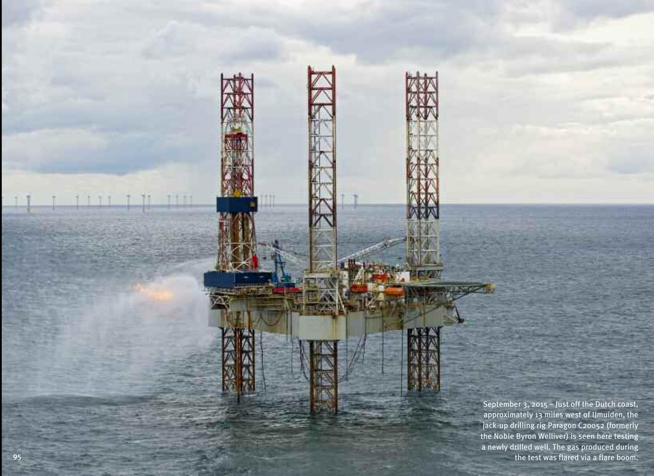
September 3, 2015 – Just off the Dutch coast, approximately 13 miles west of IJmuiden, the jack-up drilling rig Paragon C20052 (formerly the Noble Byron Welliver) is seen here testing a newly drilled well. The gas produced during the test was flared via a flare boom.
