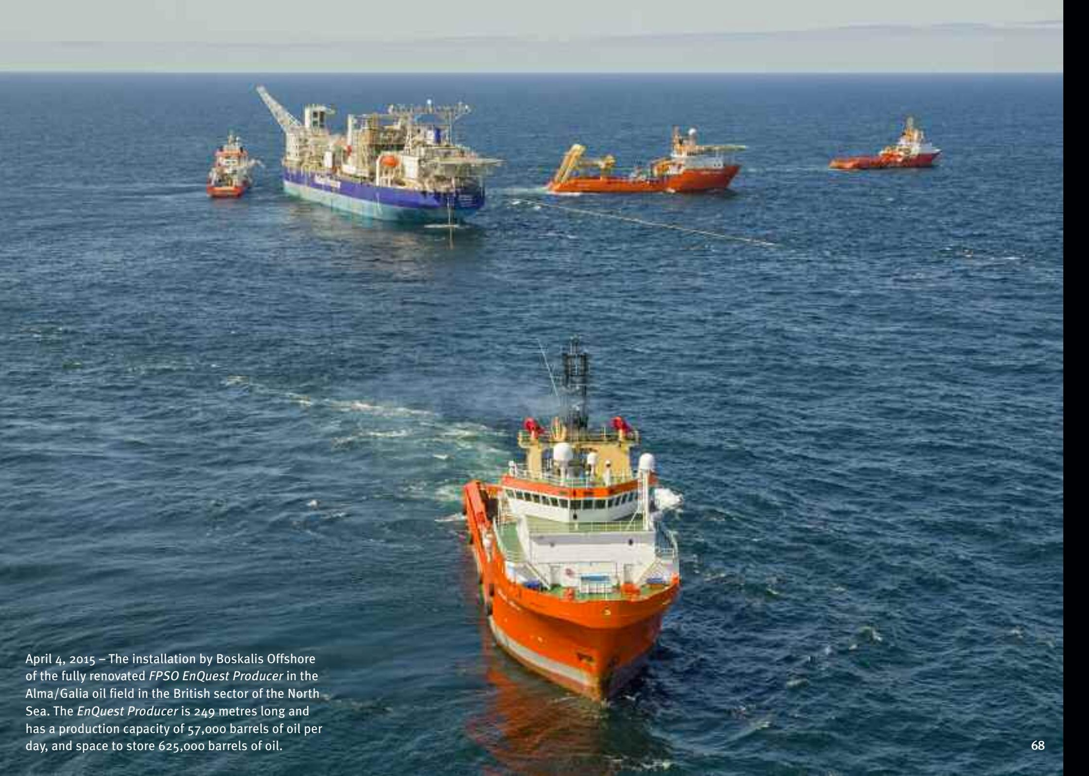
April 4, 2015 – The installation by Boskalis Offshore of the fully renovated *FPSO EnQuest Producer* in the Alma/Galia oil field in the British sector of the North Sea. The *EnQuest Producer* is 249 metres long and has a production capacity of 57,000 barrels of oil per day, and space to store 625,000 barrels of oil.
