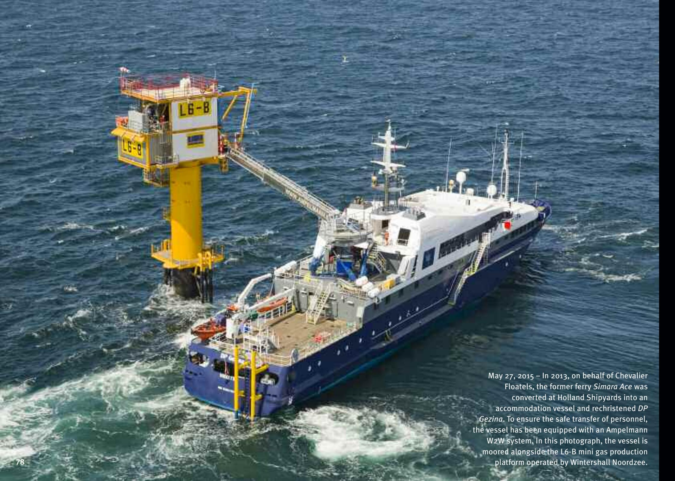
May 27, 2015 – In 2013, on behalf of Chevalier Floatels, the former ferry *Simara Ace* was converted at Holland Shipyards into an accommodation vessel and rechristened *DP Gezina*. To ensure the safe transfer of personnel, the vessel has been equipped with an Ampelmann W2W system. In this photograph, the vessel is moored alongside the L6-B mini gas production platform operated by Wintershall Noordzee.
