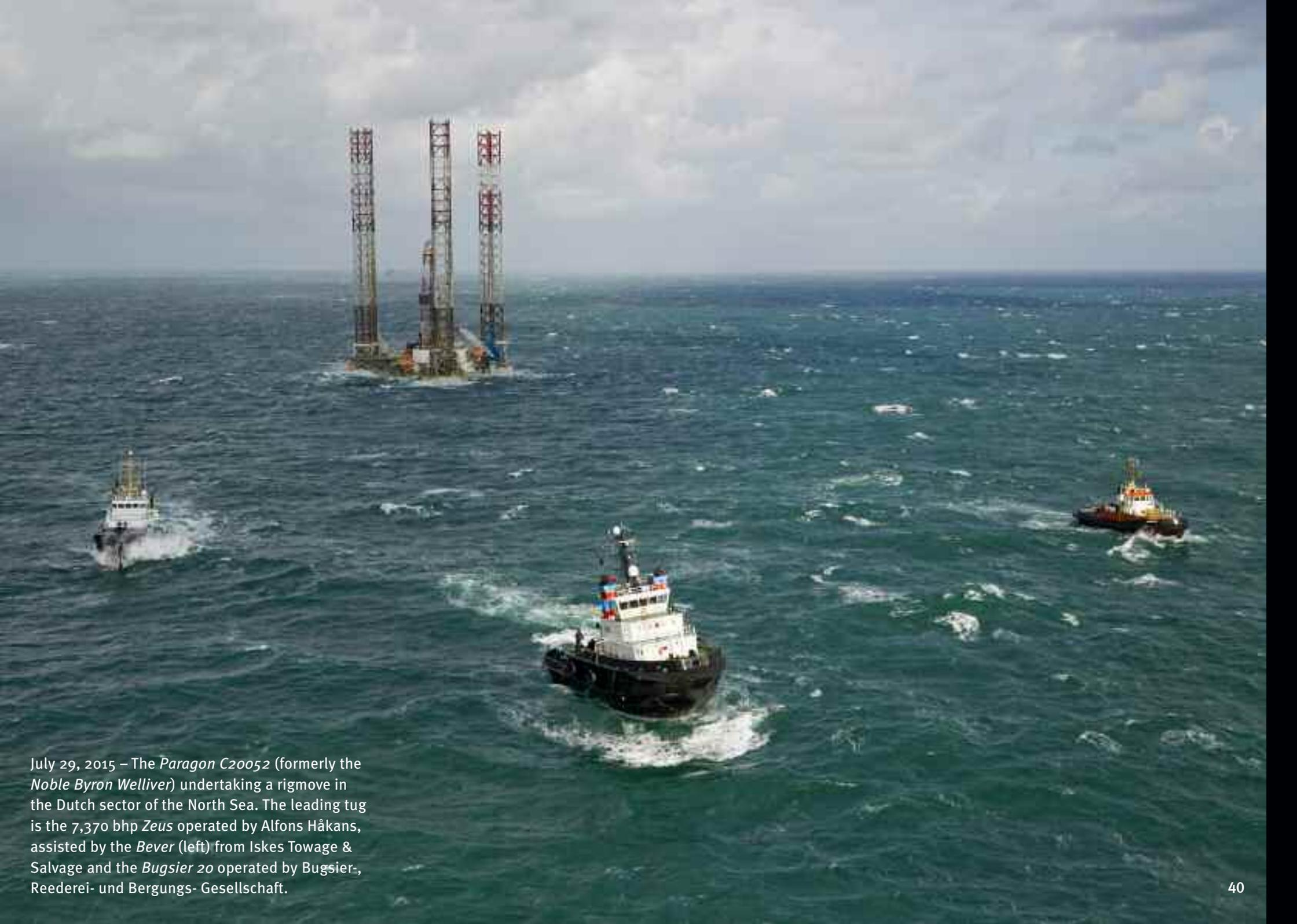
July 29, 2015 – The *Paragon C20052* (formerly the *Noble Byron Welliver*) undertaking a rigmove in the Dutch sector of the North Sea. The leading tug is the 7,370 bhp *Zeus* operated by Alfons Håkans, assisted by the *Bever* (left) from Iskes Towage & Salvage and the *Bugsier 20* operated by Bugsier-, Reederei- und Bergungs- Gesellschaft.
