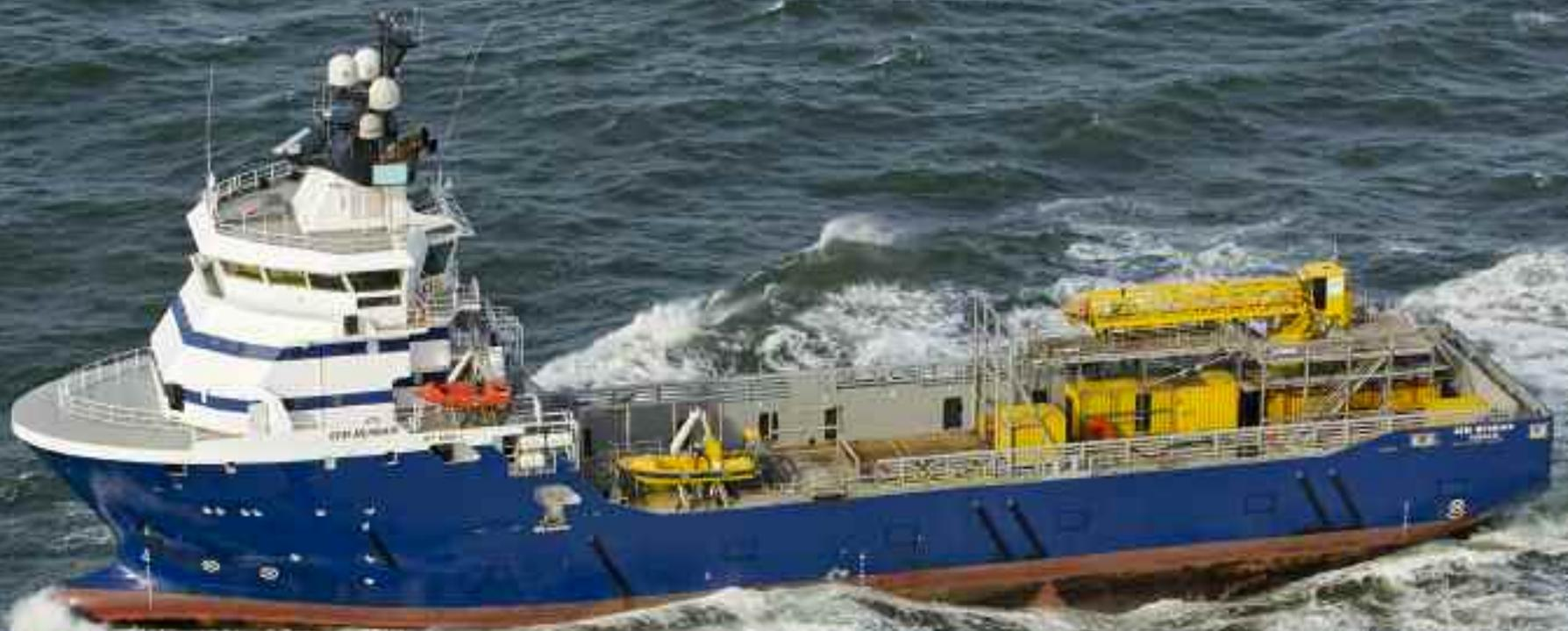
April 1, 2015 – The Norwegian supply vessel *Rem Mermaid*, operated by Rem Offshore, is deployed by GDF SUEZ E&P Nederland as a maintenance vessel for offshore platforms. To allow safe passage of maintenance personnel from a moving ship to a fixed platform, the work deck is equipped with a so-called swell compensating Offshore Access System.
