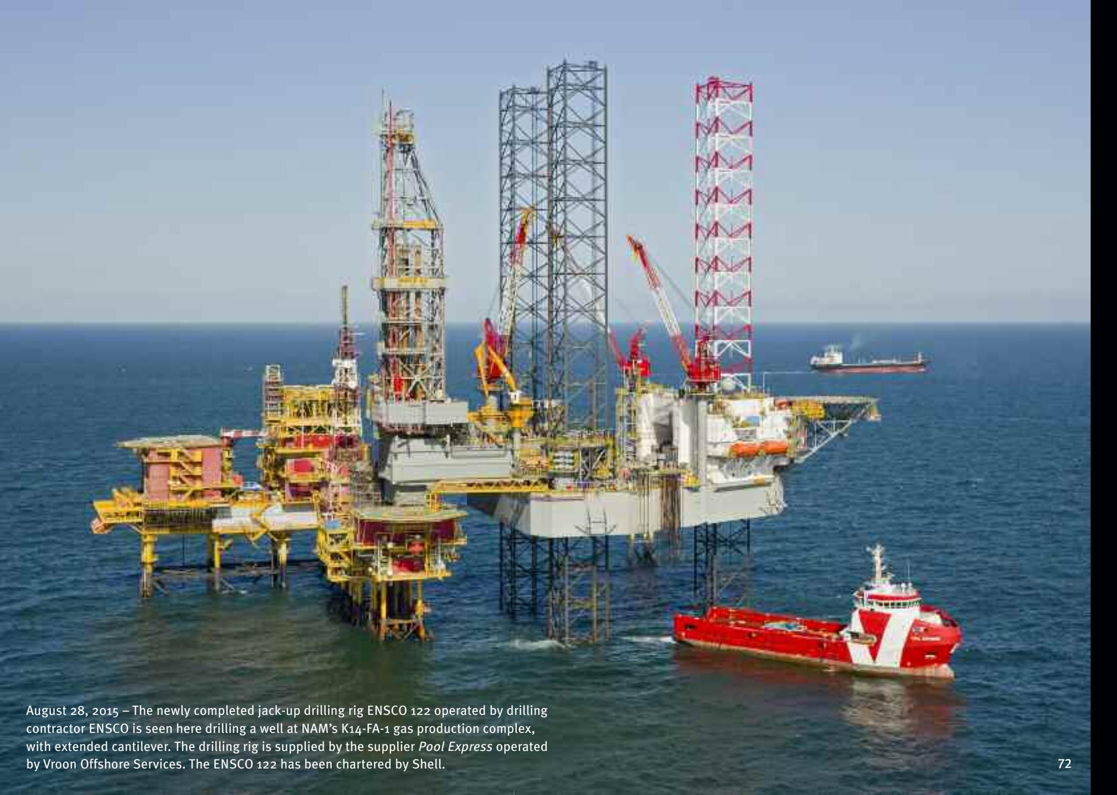
August 28, 2015 – The newly completed jack-up drilling rig ENSCO 122 operated by drilling contractor ENSCO is seen here drilling a well at NAM's K14-FA-1 gas production complex, with extended cantilever. The drilling rig is supplied by the supplier *Pool Express* operated by Vroon Offshore Services. The ENSCO 122 has been chartered by Shell.
