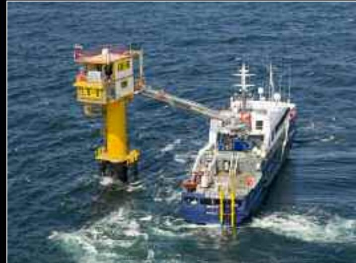
*Accommodation vessel with Ampelmann Walk-to-Work installation.*
