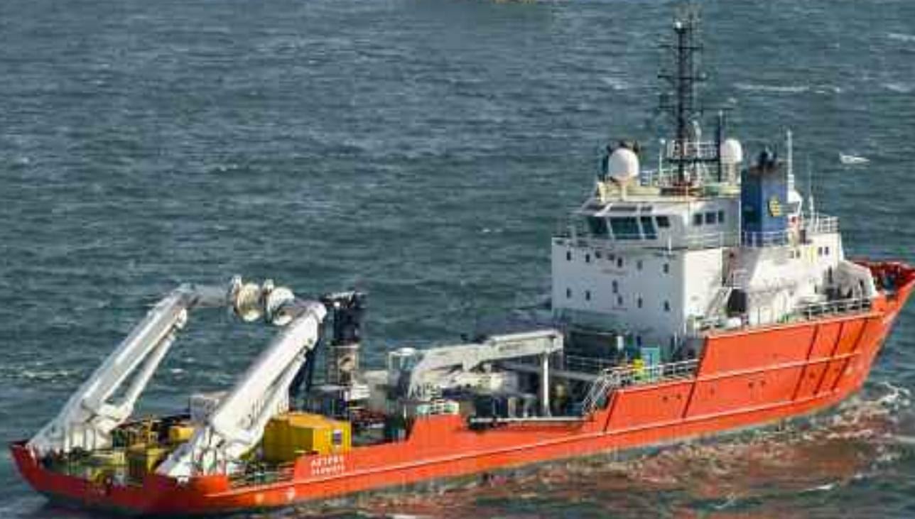
October 3, 2013 – During the laying of the pipeline between the P15 and Q13a-A platforms, the pipelay vessel *Lewek Centurion* was assisted by the dp2 multipurpose support vessel *Astrea*. For this task, the *Astrea*, chartered by N-Sea, was specially equipped with ROVs and survey equipment.
