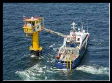
Accomodationvessel with Ampelmann Walk-to-Work installation.
