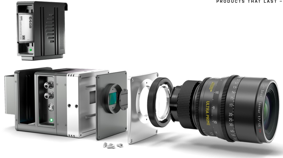
OPEN SOURCE CINEMA CAMERA Build your dream camera, one module after the other. AXIOM is an open hardware plus free software family digital of cinema camera devices. AXIOM camera systems are not only fully open but also built to be entirely modular, ready to evolve into things not even imaginable today. The Open Module Concept renders changing camera parts as easy as exchanging PCIe cards in a PC. It therefore renders AXIOM cameras to be fully extendible and keeps them from being outdated any time soon. This ensures sustainability of the entire assembly, since any module - such as the image sensor - can be replaced while keeping the rest of the camera intact.
