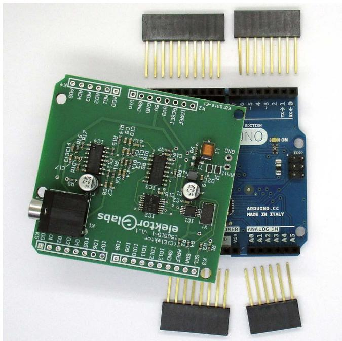
Figure 1.3: The shield and its connectors
