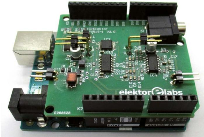
Figure 1.2: The SDR shield on an Arduino Uno
