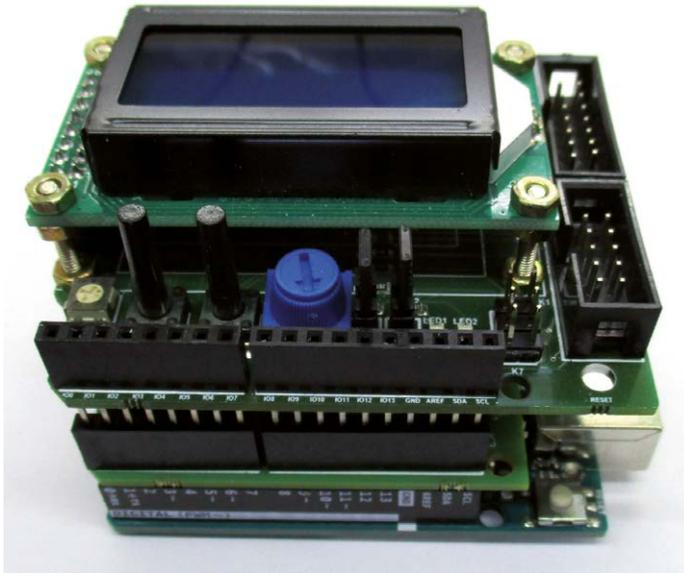
*Figure 1.9: The newer Display Shield*
