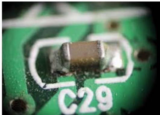
Figure 1.2: A surface-mounted component attached to a PCB.
