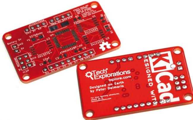
Figure 1.3: The white letters and lines is the silkscreen print on this PCB.
