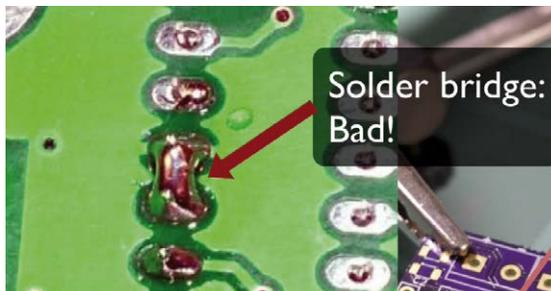
*Figure 1.5: A solder bridge like this one is a defect that solder mask helps in preventing.*
